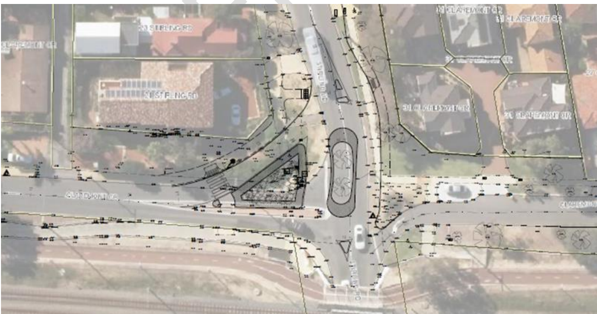
Figure 7-40 Stirling Road / Claremont Crescent – modified 'roundabout'
