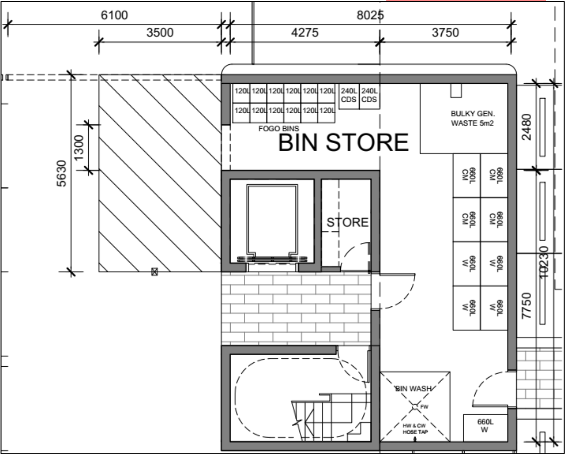
Figure 4: Basement bin store layout
