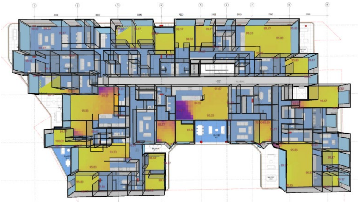
Figure 9: Daylighting for Sixth Floor to Seventh Floor
